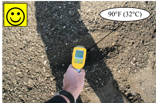
Figure 6.23: Recycled material (warm, good dispersion).
