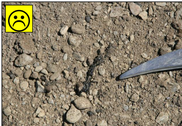
Figure 6.13: Unfoamed binder in recycled material.
