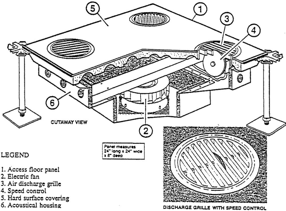
**Figure 1. Floor Supply Module**
