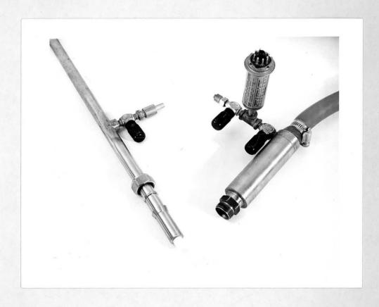
Figure 2. Close up of Teflon seal on straight section and coupling on flexible receiver end.
