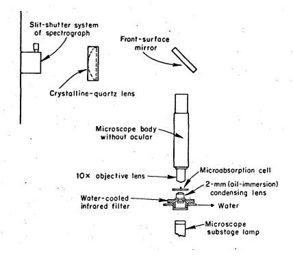
FIG. 4. Apparatus used to record absorption spectra on a grating spectrograph.
