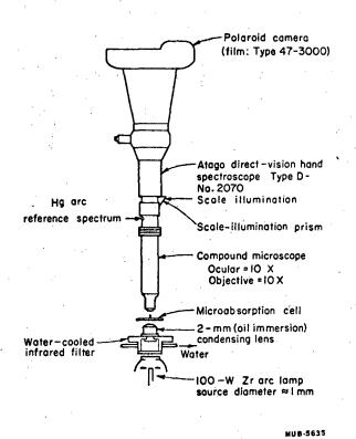
FIG. 2 Apparatus for photographing spectra through a hand spectroscope.
