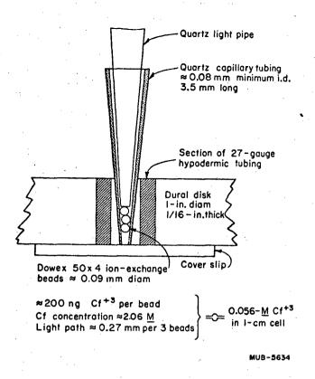
FIG. 1 Stacked bead microabsorption cell.
