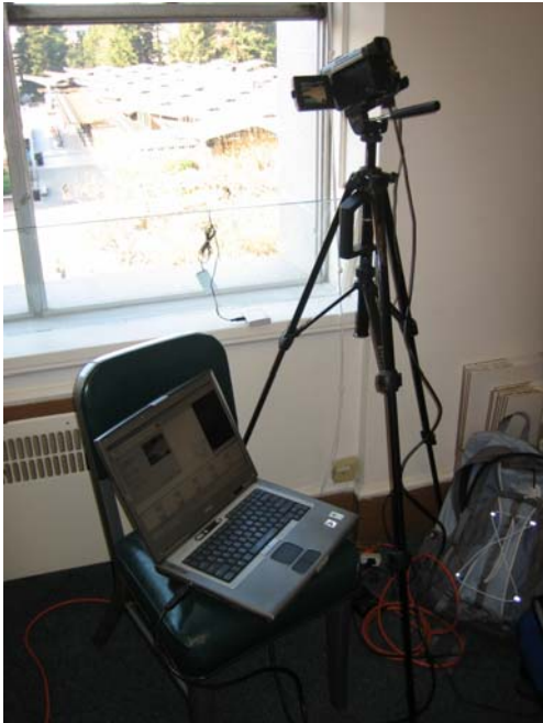
Figure 3.9 Recording setup. A digital video camera is connected to a laptop and a Hobo data logger (at the window) collects temperature and relative humidity.
