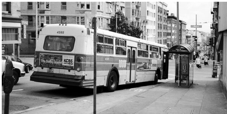
Figure 6. Bus loading zone that is shorter than the overall length of the bus.
