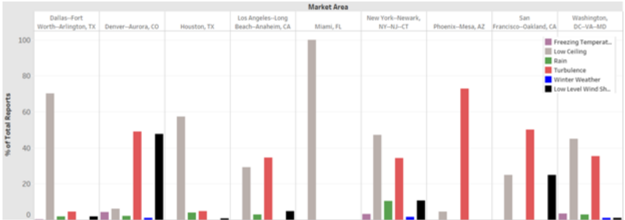
Figure 2: Distribution of PIREPs by weather condition at focus urban areas. No PIREPs were generated across our historical period in Honolulu
