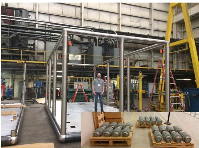
FIG. 7. High voltage platform shown after fabrication with insulator shown in bottom insert.
