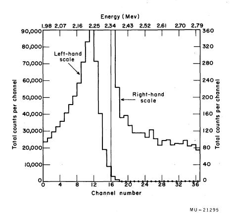
Fig. 1. Alpha particle spectrum of "enriched Sm 146" sample.
