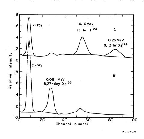
Fig. 1. Typical low-energy photon spectra from I samples on the (A) second and (B) third day after bombardment.
