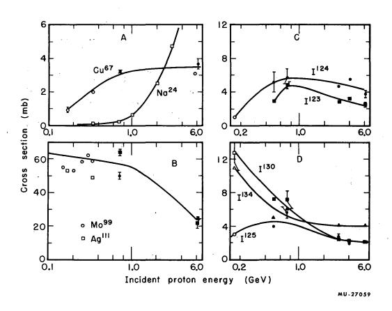
Fig. 2. Excitation functions for some representative nuclides. The solid points are from this work. The open points are from reference 14.
