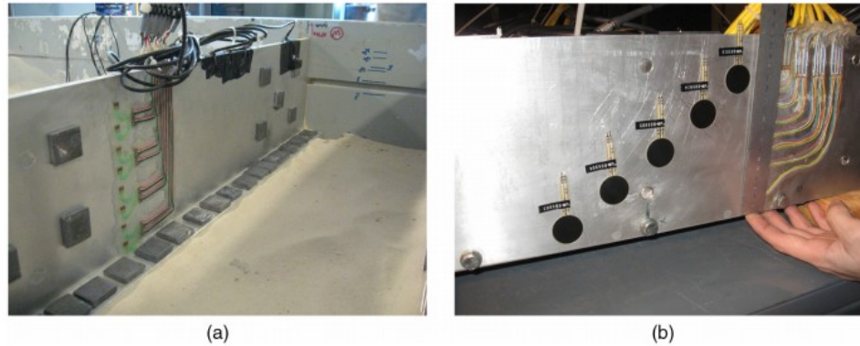
Fig. 2. (a) Strain gauges located at the walls of the retaining structures; (b) pressure transducers placed on the sides of the retaining structures
