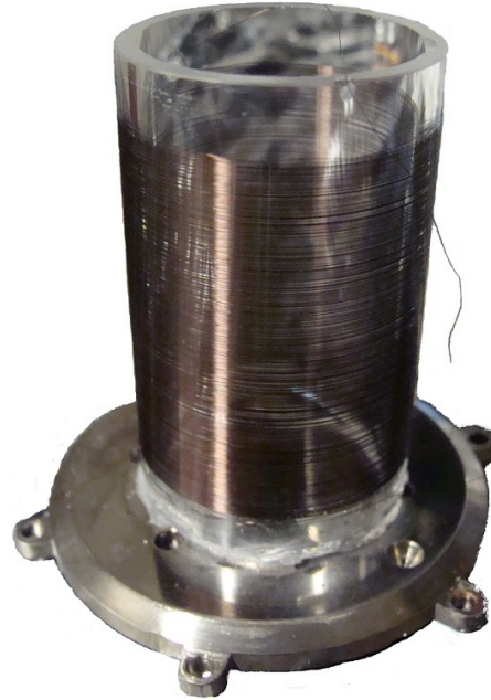
Figure 6.5: Picture of a finished coil. Nb wound on a quartz cylinder.
