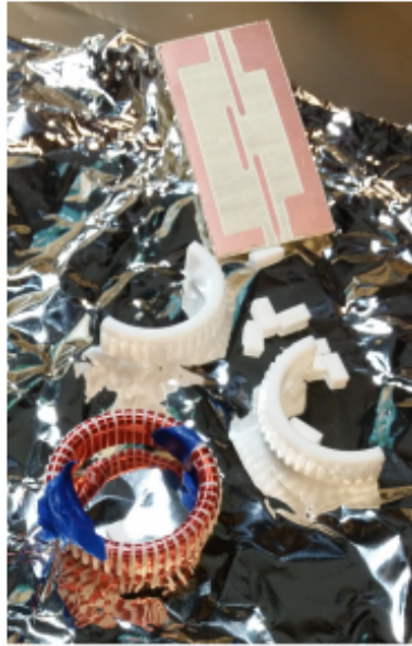
Figure 6.12: Picture of a toroidal resonator and the PTFE parts used as a former. This specific resonator is wound from copper wire while the ones in our experiment are made from NbTi wire.
