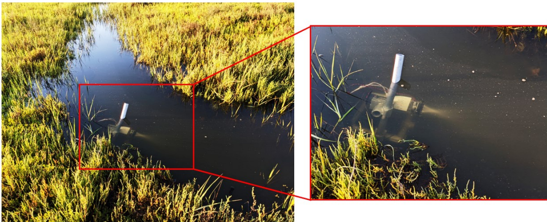
Supplementary Figure 3.5: The field deployment of the system in a water channel at the Kendall-Frost saltmarsh, San Diego, California. The instrument was mounted on an aluminum speed rail structure that lifted the system approximately 0.3 m above the bottom of the channel. The inset shows the converging light from the LEDs that was collimated by the Fresnel lens.
