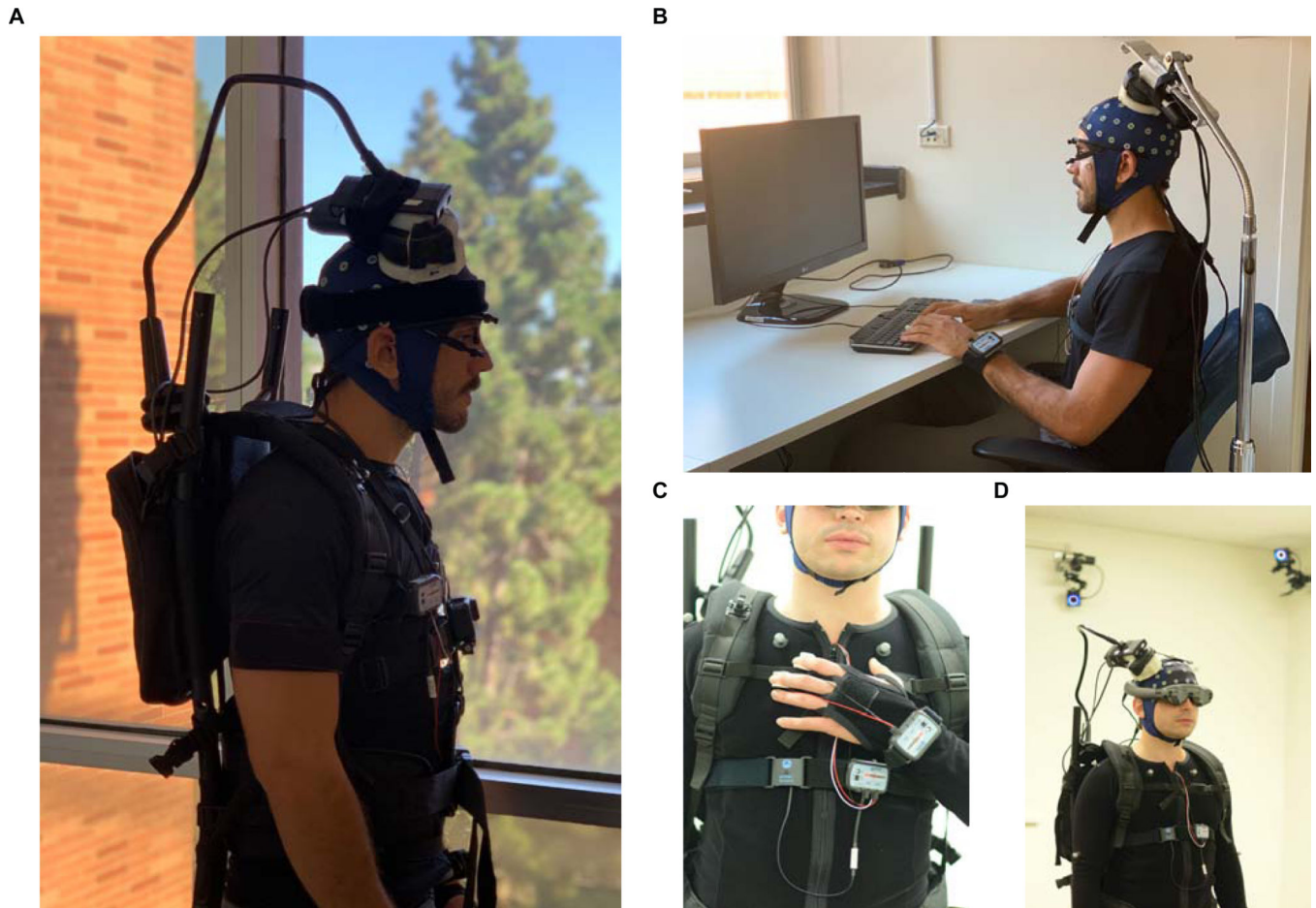
Figure 6. Additional photos of the Mo-DBRS platform in naturalistic and laboratory settings (A) A participant wearing the Mo-DBRS Full platform showing the backpack connected to the Wand. (B) A participant performing a laboratory-based stationary task. (C) Wearable equipment for biometric recordings, including a respiration belt, skin conductance and heart rate sensor. (D) A participant wearing the Mo-DBRS Full platform with the Magic Leap AR headset in a laboratory equipped with wall-mounted motion capture cameras.
