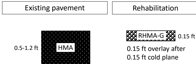
Figure 2.6: VEN-1 pilot rehabilitation.
