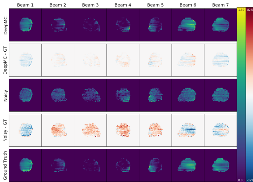
Figure 5-10. Plan delivery parameters (X-ray beamlet fluence) for the first testing patient resulting from optimization using DeepMC, high-, and low-noise beamlet dose. All color scales are consistent, and limits are shown in the color bars on the right. All are normalized to the per-beam maximum fluence from the ground truth plan.
