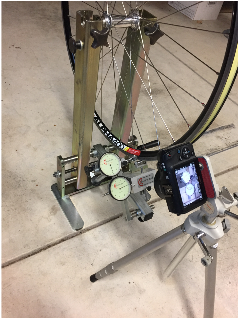
Figure 2.3: Measurement setup of the Centrimaster truing stand, digitization camera and tripod. The test wheel used for all the experiments is mounted in the truing stand. Not shown is the WheelFanatyk tensiometer used to measure spoke tension.
