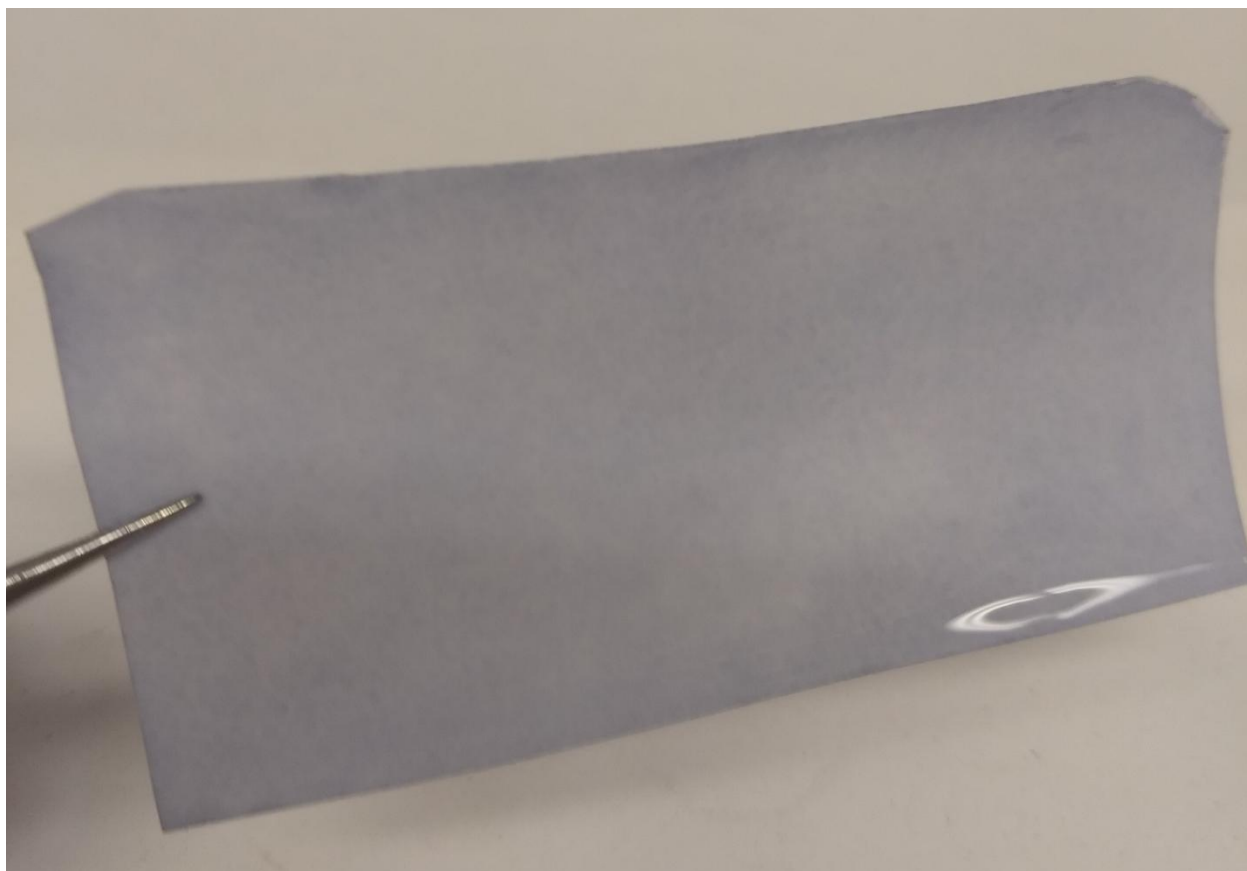
Figure S6-3. Photo showing a modified PES membrane which has been kept in water for almost one year.
