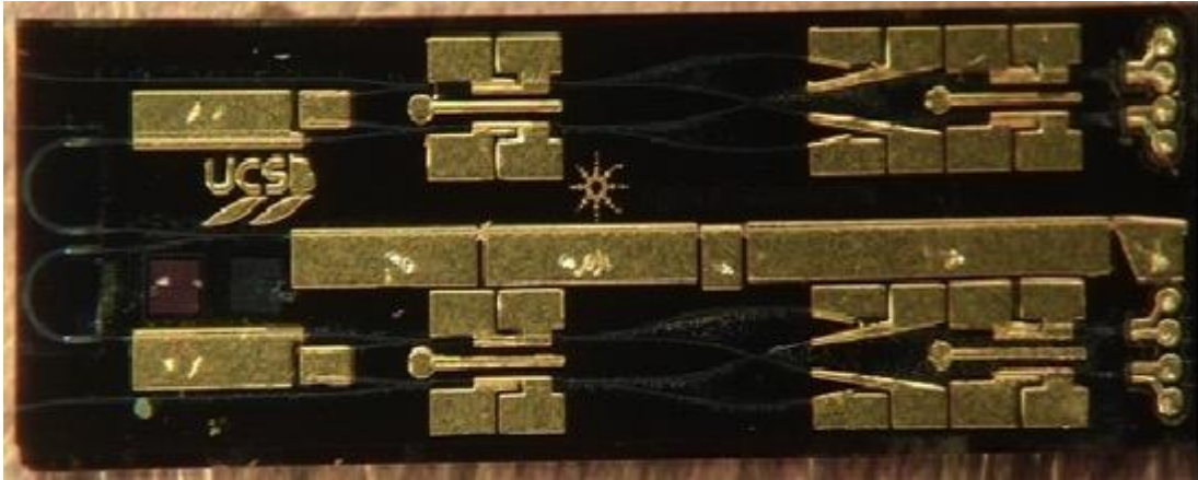
Figure 7.2. Image of the fabricated dual channel coherent receiver. Reprinted with permission from [78].
