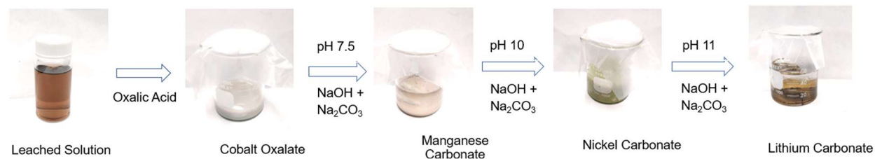
Figure 9. Schematic illustration of metal salt extraction process
