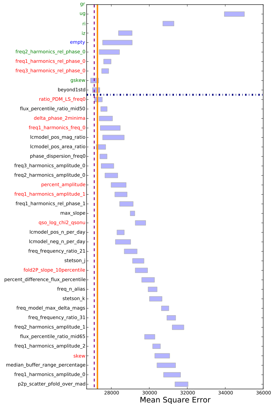
Figure 7.9: Results of the forward feature selection process for T_{\text{eff}} . We begin by selecting g - r ( gr in the figure) and iteratively add the feature that most improves the regression model as measured by the improvement in the FoM. Boxes show the cross-validated range of MSE following the addition of the feature to the model. The vertical dashed line shows the minimum MSE, while the vertical orange line shows the threshold FoM (minimum + 1\sigma ). Features above the dash-dot line are those that are selected for the optimal feature set. The procedure was rerun 5 times and the feature names are color coded according to the number of times they were selected in the optimal feature set: 0 (black), 1 (red), 2 (blue), 3+ (green). For brevity, only the first 40 selected features are shown.
