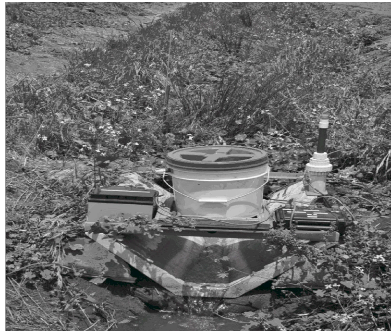
Figure 14. Anderson trial showing vegetative ditch and electronic dosing unit, 2008. Photo by B. Anderson
