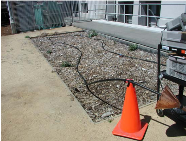
Figure 10. The setup for a frequency scan with the cable completely placed on the ground, with the exception of the sections around the sending and the receiving funnels, which have to be elevated to avoid deforming the funnel geometry.
