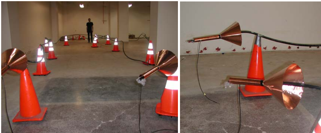
Figure 2. The 90 foot in-lab underground cable GW setup. The cable was elevated on ten 29 inch tall plastic traffic cones, to avoid the interaction of the wave with the reinforced concrete floor underneath.
