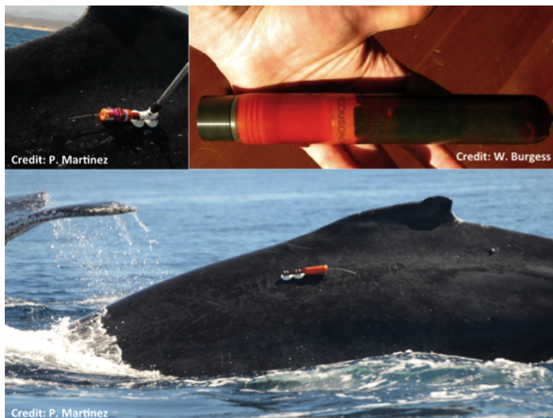
Figure 4.2: The Acousonde (top right) and B-probe look similar, and are both attached to the whale using a tagging pole (top left). Suction cups hold the tag on the whale's body for a few hours while an orange buoy and VHF antenna (bottom) keep it above water for recovery once it fell off the whale.
