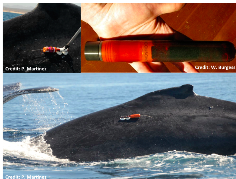
Figure 1.5: Three views of the Acousonde by Greeneridge Sciences, Inc. used in this dissertation: top right is the tag itself to the scale of a human hand, top left depicts the attachment method of the tag encased in a buoy with suction cups, and the bottom shows the scale of the tag to the size of a humpback whales body.
