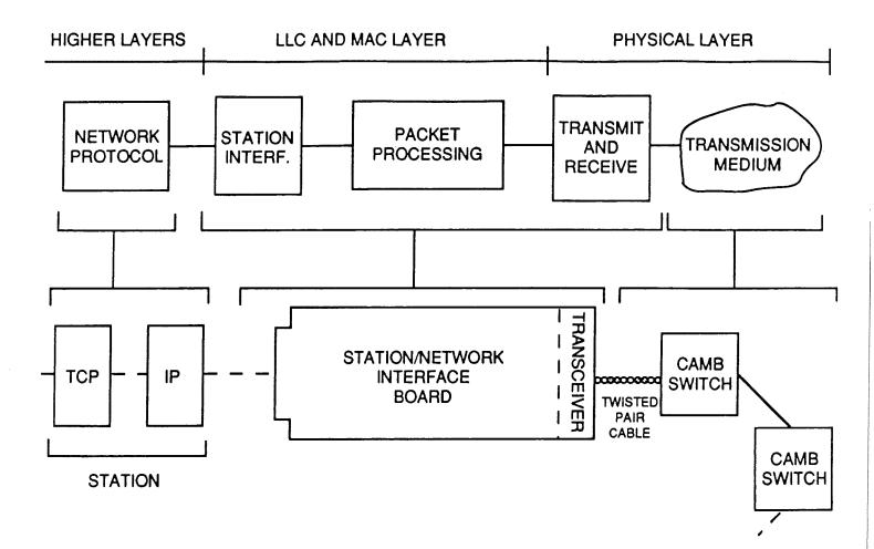
Figure 2: Layering Architecture of the CAMB Tree
