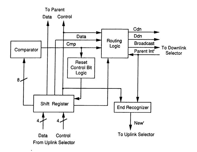
Figure 7: Address Recognizer Block Diagram
