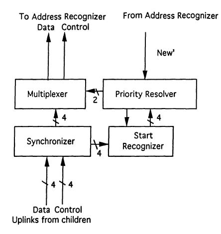
Figure 6: Uplink Selector Block Diagram
