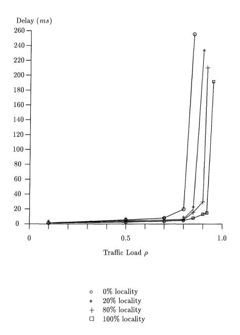
Figure 19: Transmission Delay in a 2-Level CAMB Tree
