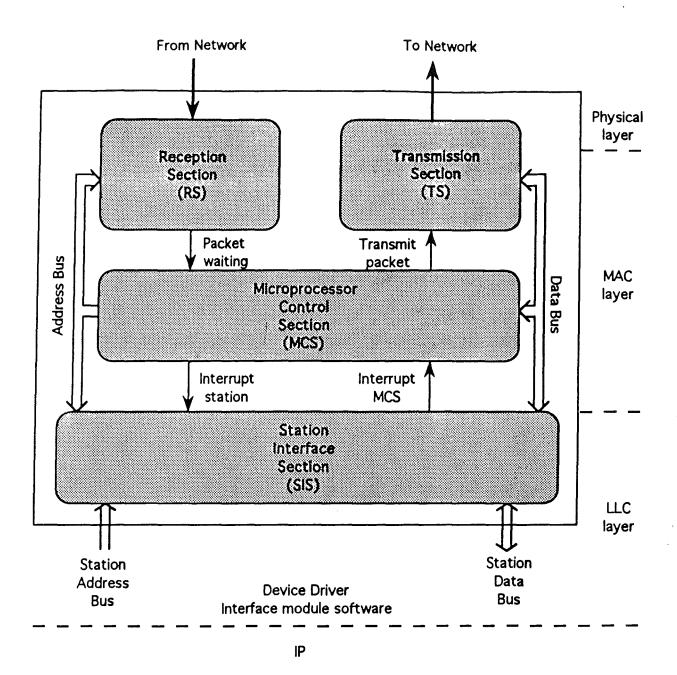
Figure 9: Station/Network Interface Board
