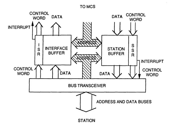
Figure 10: Station Interface Section Block Diagram
