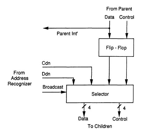
Figure 8: Downlink Selector Block Diagram
