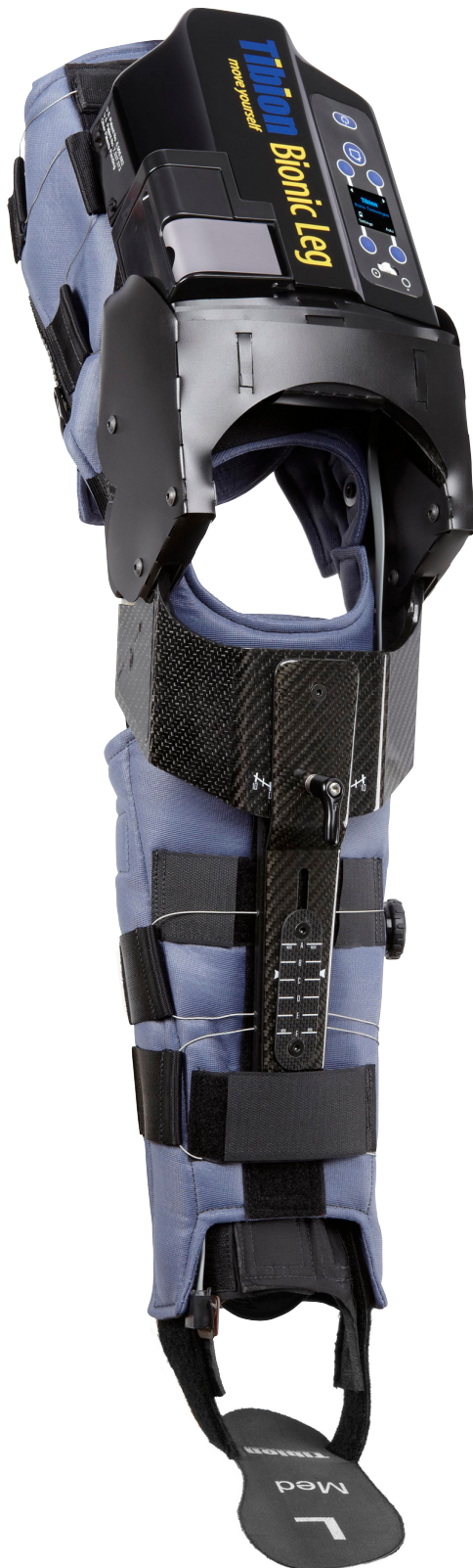
Figure 1 Robotic leg orthosis. (a) Tibion Bionic Leg orthosis and (b) shoe insert with foot sensor.
