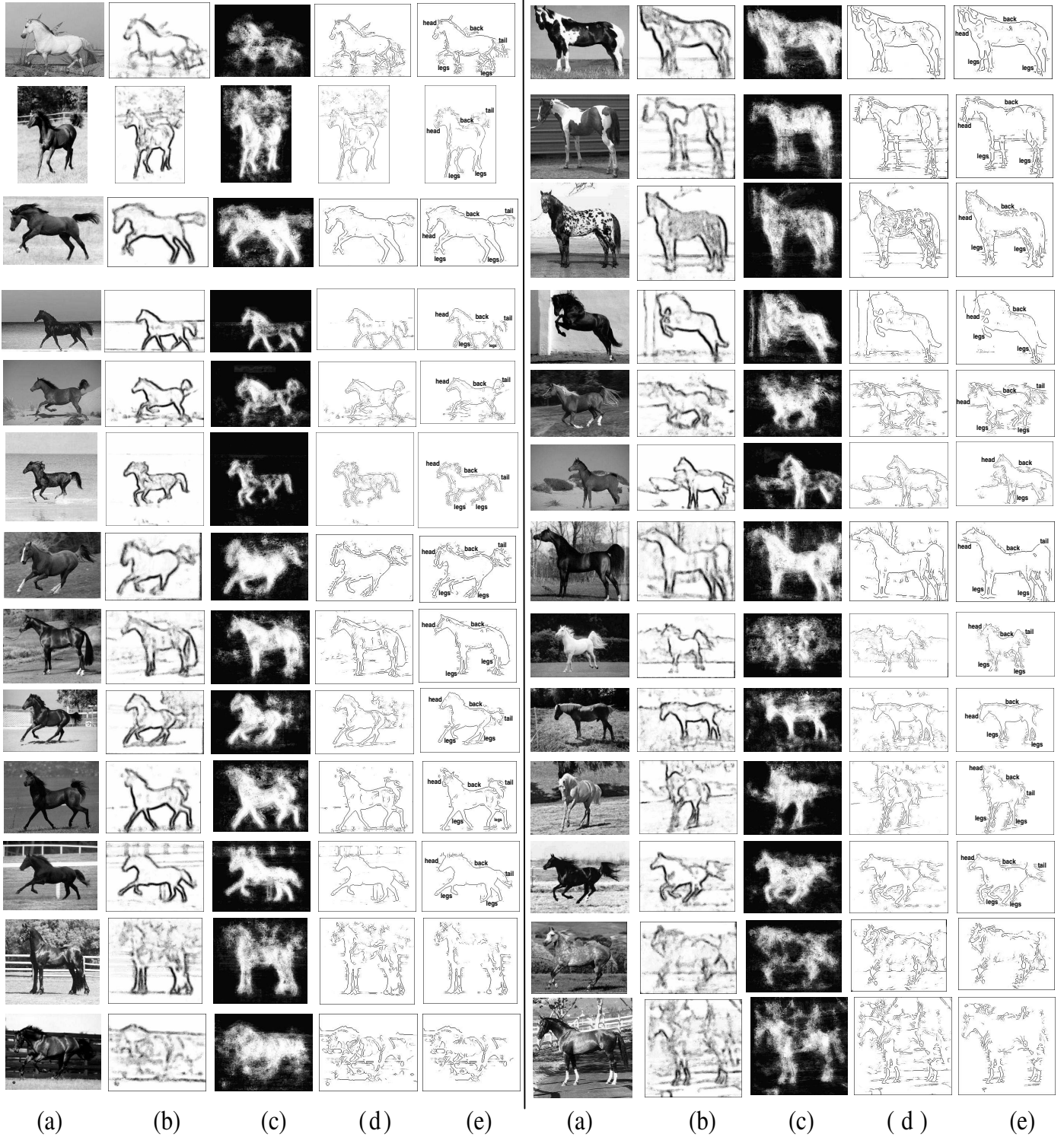
Figure 8. Results on some testing images. (a) shows input images in gray scale. (b) are the boundary maps detected by BEL. (c) shows the body maps. (d) demonstrates refined boundaries based on the short-range context information. (e) gives final results after shape matching, and also the different parts of the horses are labelled according to the shape matching results. These images are representatives of the data set, which have different appearances, poses, scales, and lightening conditions. We see how each level of information is helping detecting their boundaries. The last two rows in both the columns show two worst results by our algorithm.
