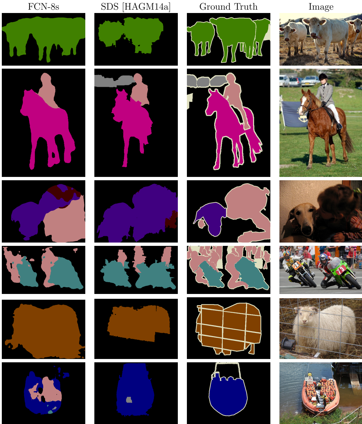
Figure 3.6: Fully convolutional segmentation nets produce state-of-the-art performance on PASCAL. The left column shows the output of our highest performing net, FCN-8s. The second shows the segmentations produced by the previous state-of-the-art system by Hariharan et al. [HAGM14a]. Notice the fine structures recovered (first row), ability to separate closely interacting objects (second row), and robustness to occluders (third row). The fourth row shows a failure case: the net sees lifejackets in a boat as people.
