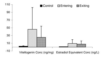
Figure 3. Estradiol equivalent concentrations estimated by yeast estrogen screening assay of wastewater samples from the Green Acres Plant and Prado Wetland.
