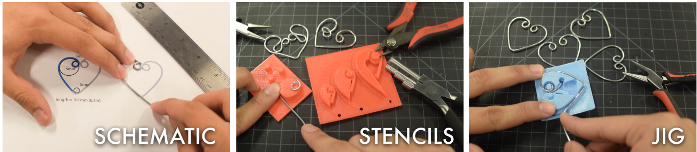
Figure 1. a) Schematic, an annotated construction proxy used to provide fabrication feedback, b) Stencil, a fabrication proxy that breaks down designs into elementary forms, c) Jig, a fabrication and construction proxy that provides a ritual high-fidelity fabrication process.
