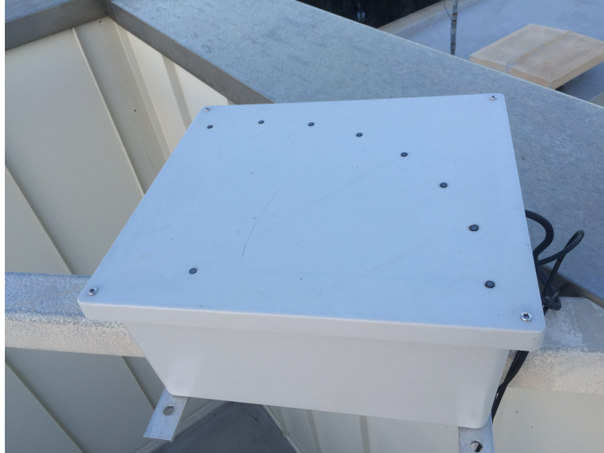
Figure 3.1: Cloud Shadow Speed Sensor (CSS) contained inside a weather-proof enclosure with dimensions 0.45 x 0.40 m. On the top of the enclosure is an array of nine phototransistors.
