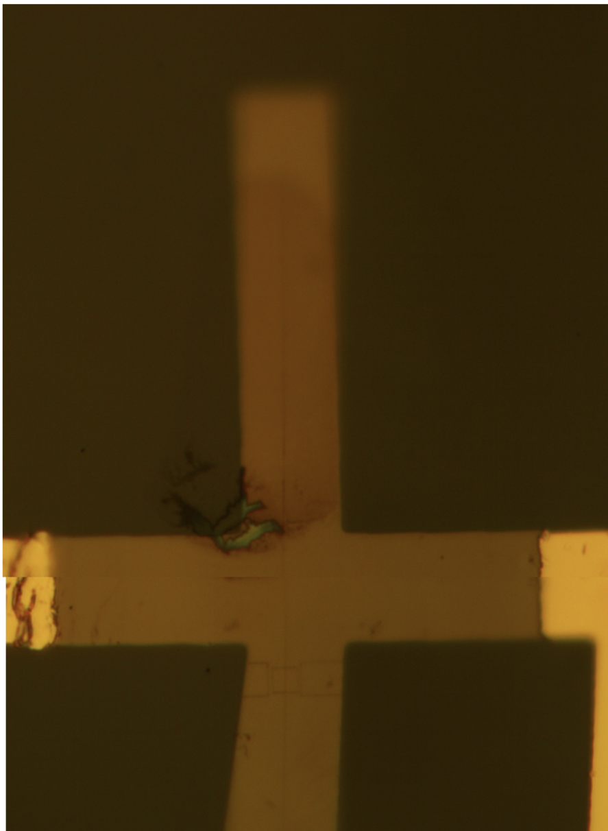
Figure 6.13: Close up optical image of focused HeIB directly written SQUID. The faint lines are created by ion beam induced disorder and make up the Josephson Junctions, squid loop and additional lines to shorten the width of the junction.
