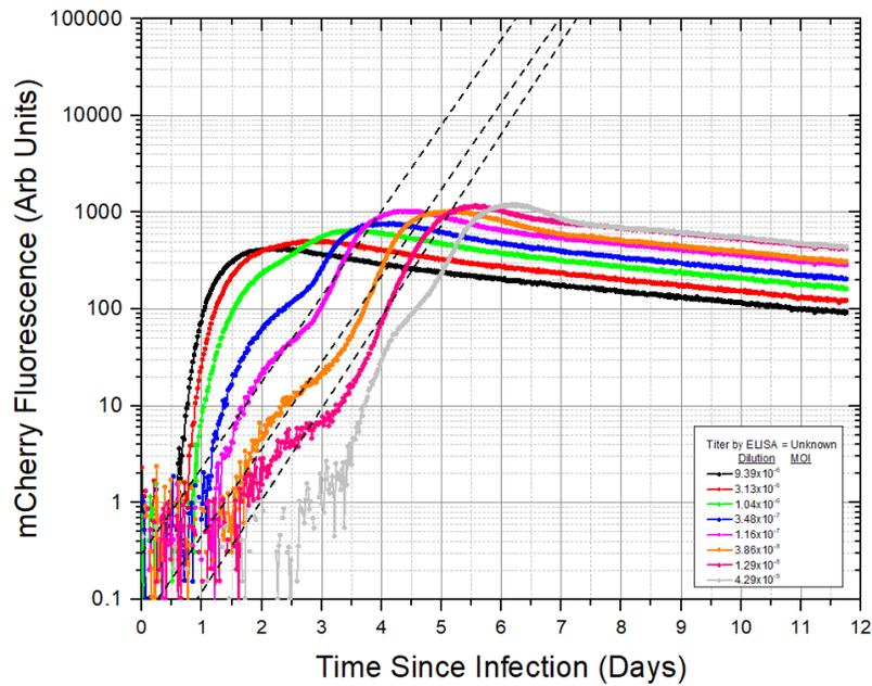
Figure 2.12. Measured fluorescence signal vs. time for PMCN-871 (mCherry-P2A-ADP) infecting A549 cells. The lower signal levels and higher noise values are a result of the lower quantum efficiency of mCherry compared to YPet. The resulting ln-slope is  $2.10 \text{ days}^{-1} (+0.08/-0.06)$ .
