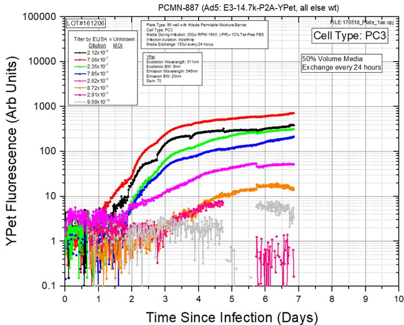
Figure 3.7. Kinetics curves for Ad5 wt (Ad5 5/5/5, PCMN-887) when infecting PC3 cells with 50% volume media exchange every 24 hours. Note the stall in fluorescence growth near the end of each 24 hour period with rapid increase following media exchange (red and black curves).
