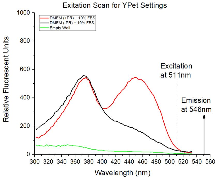
Figure 2.4b. Measured fluorescence spectrum for DMEM media at YPet emission peak.
