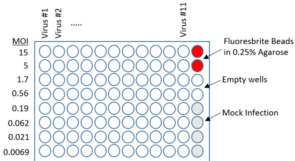
Figure 2.10. Layout for FVBK assay. 11 different viruses can be monitored on a single 96 well plate. The 12<sup>th</sup> column of wells is used for normalization constant, empty wells for later WST-1 cell viability assay, and Mock infected wells for background subtraction.
