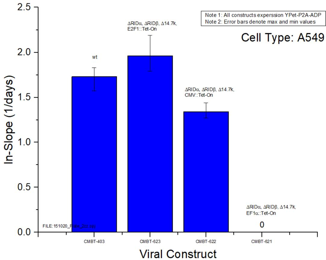
Figure 4.4. Measured replication kinetics of virus constructs with Tet-On gene placed in the E3B region of Ad5 genome.
