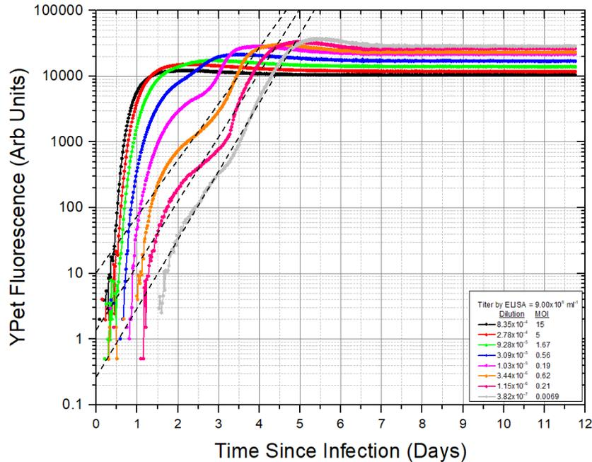
Figure 2.11b. Same data as shown in Fig 2.10a, but plotted on a semi-log graph for PCMN-421 (YPet-P2A-ADP). The dashed lines show the fits to the logarithmic growth portion of the curves with a resulting ln-slope of  $2.20 \text{ days}^{-1}$  (+0.20/-0.23)
