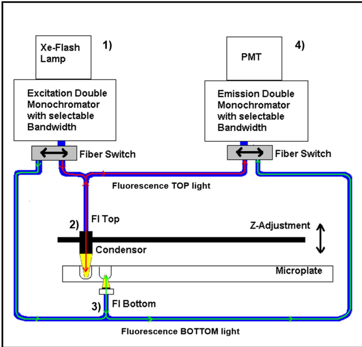
Figure 2.7. Optical layout of TECAN plate readers (figure taken from Infinite M1000Pro users manual).
