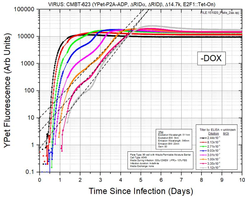
Figure 4.6b. Measured YPet fluorescence versus time for construct with E2F1 promoter driving Tet-On ORF located in the E3B region.
