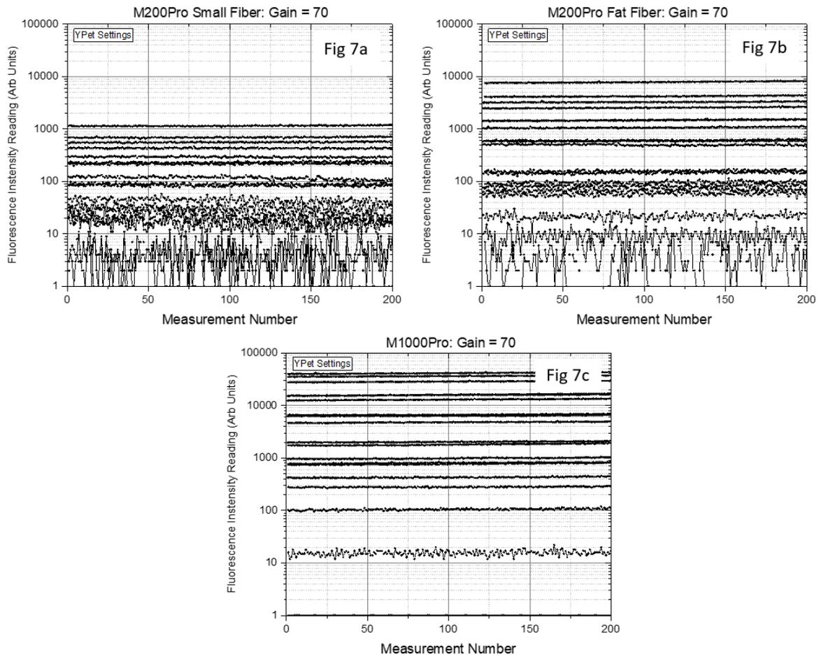
Figure 2.8. Measured fluorescence intensity for a dilution series of fluorescent beads suspended in agarose. 200 measurements made for each fluorescent bead dilution. Plate reader type: a) M200Pro, b) M200Pro with fat fiber, c) M1000Pro.
