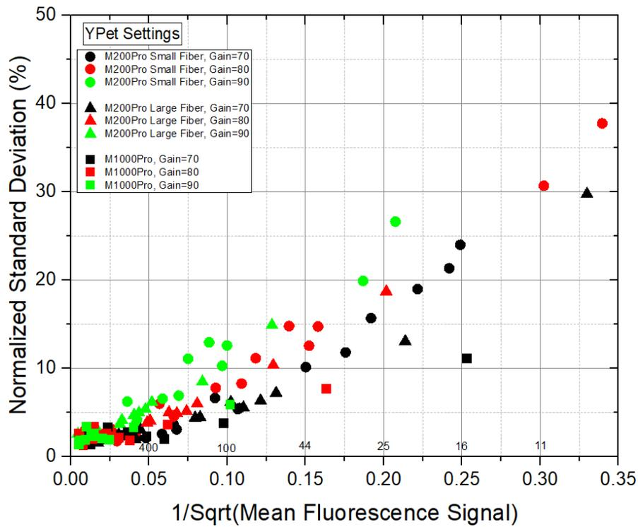
Figure 2.9. Normalized standard deviation of measured fluorescence intensity vs. square root of measured fluorescence for each instrument.
