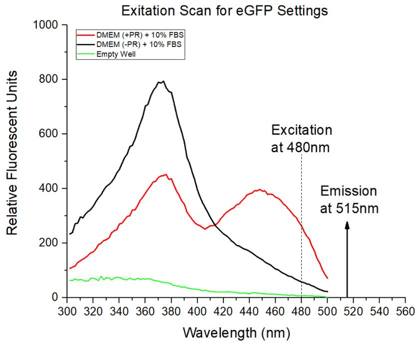
Figure 2.4a. Measured fluorescence spectrum for DMEM media at eGFP emission peak.
