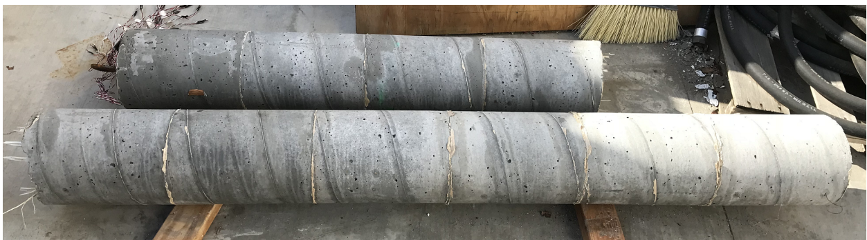
Figure 3.50: Pile 2: Cracked pile.
