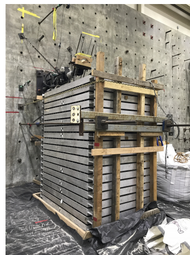
(b) Reinforced wooden bracing.
