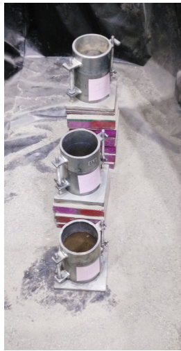
(a) Proctor molds used during the calibration
