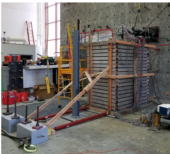
(a) Initial wooden bracing.
