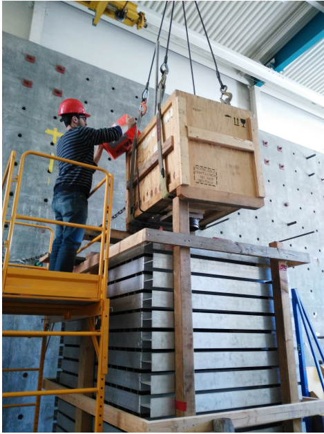
(a) Pluviator attached to the crane
