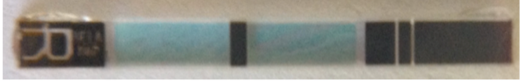
Figure 4.3: An optical image of the MAP after it has been fabricated, bonded, and diced. The blue regions correspond to the sections in which the top and bottom halves of the MAP are aligned. In the experiment described in section 4.2.2, electrons traverse these blue "accelerating regions" from the bottom of the figure to the top. The IR laser is incident into the page. The black regions correspond to the sections of the MAP sample onto which the metallic spacers were deposited.
