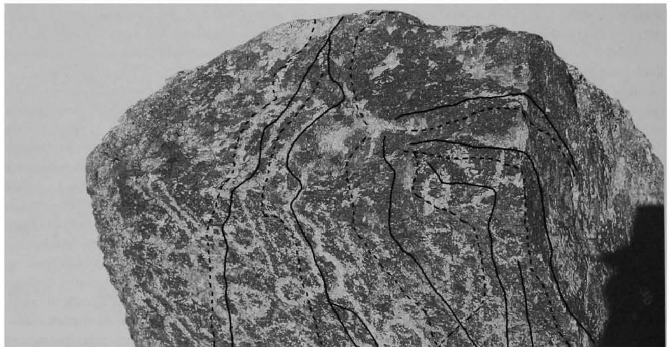
Figure 10. Lightning Rock. Lightning discharge paths on the top surface, mapped using a magnetometer (see text). Symbols as in Figure 9.
