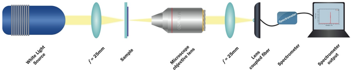
Figure 4. The free space optical setup to study the transmission of the thin film of CLC.
