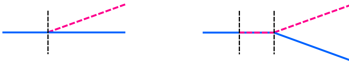
Figure 7.7: SDK beamsplitter. The initial spin state |a\rangle is shown in solid blue lines and the other spin state |b\rangle is shown in dashed red lines. The horizontal (vertical) axis is time (position), so a state's momentum can be inferred from the slope of the line showing its path. Each operation is shown with a dashed black vertical line. The left schematic shows a standard 2\hbar k Raman \frac{\pi}{2} pulse. The right shows a two-step SDK beamsplitter, where the spin-superposition and momentum-entanglement are performed in separate steps.
