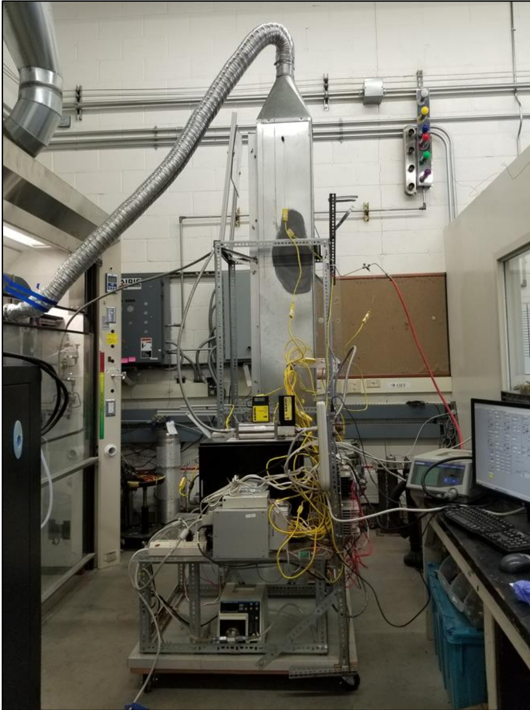
Figure 5.2: Combustion chamber and experimental facility
