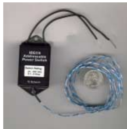
Figure 1. First prototype of the Title 24 wall switch built according to original specifications.
