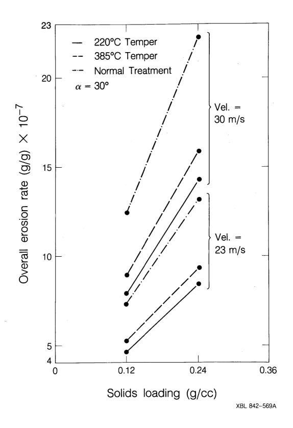
Fig. 8 Erosion rate v.s. solids loading for three tempers of steel.
