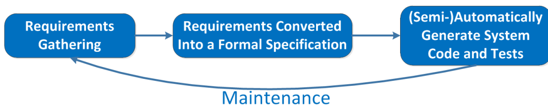
Figure 1.2. Steps in Model Driven Development [11]. The development moves from one phase to the other in one direction. If requirements change, the process starts from the beginning. Different from the Waterfall Model [127], the system code and tests are automatically or semi-automatically generated from the formal requirements specification.
