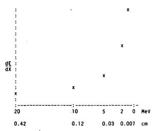
Fig. 2. Relative energy loss vs kinetic energy in MeV and range in centimeters for protons in water as  $\beta$  goes to zero.
