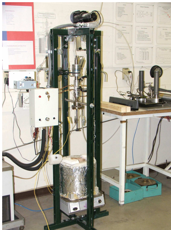
Figure 3.1 Simplified schematic diagram and photograph of the batch reactor setup
