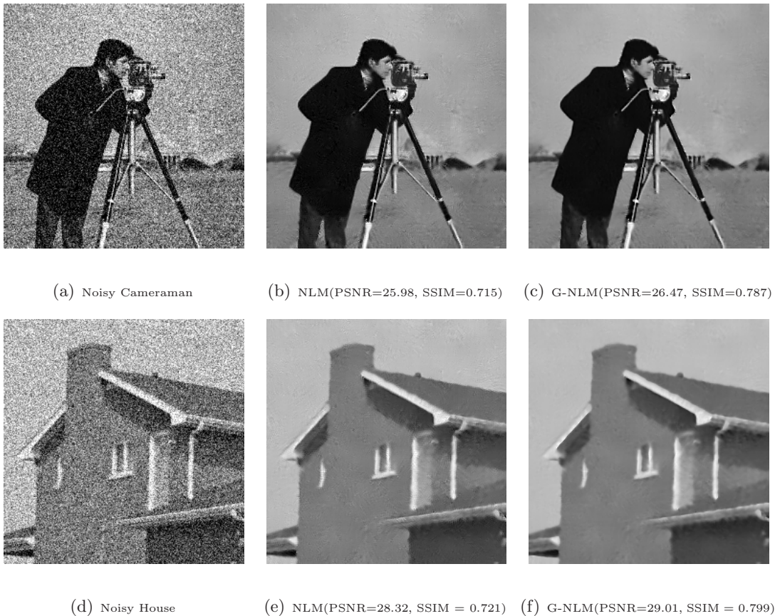
Figure 4.5: Comparison of denoising performance on noisy images corrupted by AWGN of \sigma = 40 . (a),(d) Noisy input, (b),(e) NLM [2], (c),(f) G-NLM.
