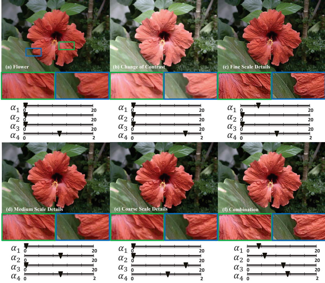
Figure 6.7: Contrast and detail manipulation of the flower image. (a) Input image, (b) \alpha_1 = 1, \alpha_2 = 1, \alpha_3 = 1, \alpha_4 = 1.5 , (c) \alpha_1 = 5, \alpha_2 = 1, \alpha_3 = 1, \alpha_4 = 1 , (d) \alpha_1 = 1, \alpha_2 = 10, \alpha_3 = 1, \alpha_4 = 1 , (e) \alpha_1 = 1, \alpha_2 = 1, \alpha_3 = 15, \alpha_4 = 1 , (f) \alpha_1 = 3, \alpha_2 = 5, \alpha_3 = 10, \alpha_4 = 1.1 .
