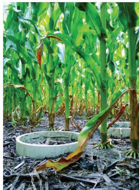
Polyvinylchloride rings are installed to facilitate GHG measurement in a corn field site in Iowa.
