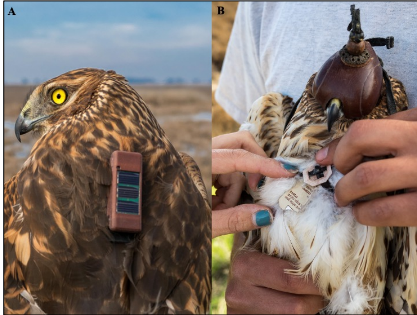
Figure 2.2. Ornitela transmitter on an adult female Northern Harrier (A), and Teflon cross-breast “X” harness design with leather patch to stabilize harness at the top of the keel (B). Photo credit: Shannon Skalos.
