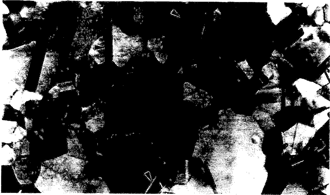
Fig. 5.1 TEM of the Microstructure of Polycrystalline Silicon
