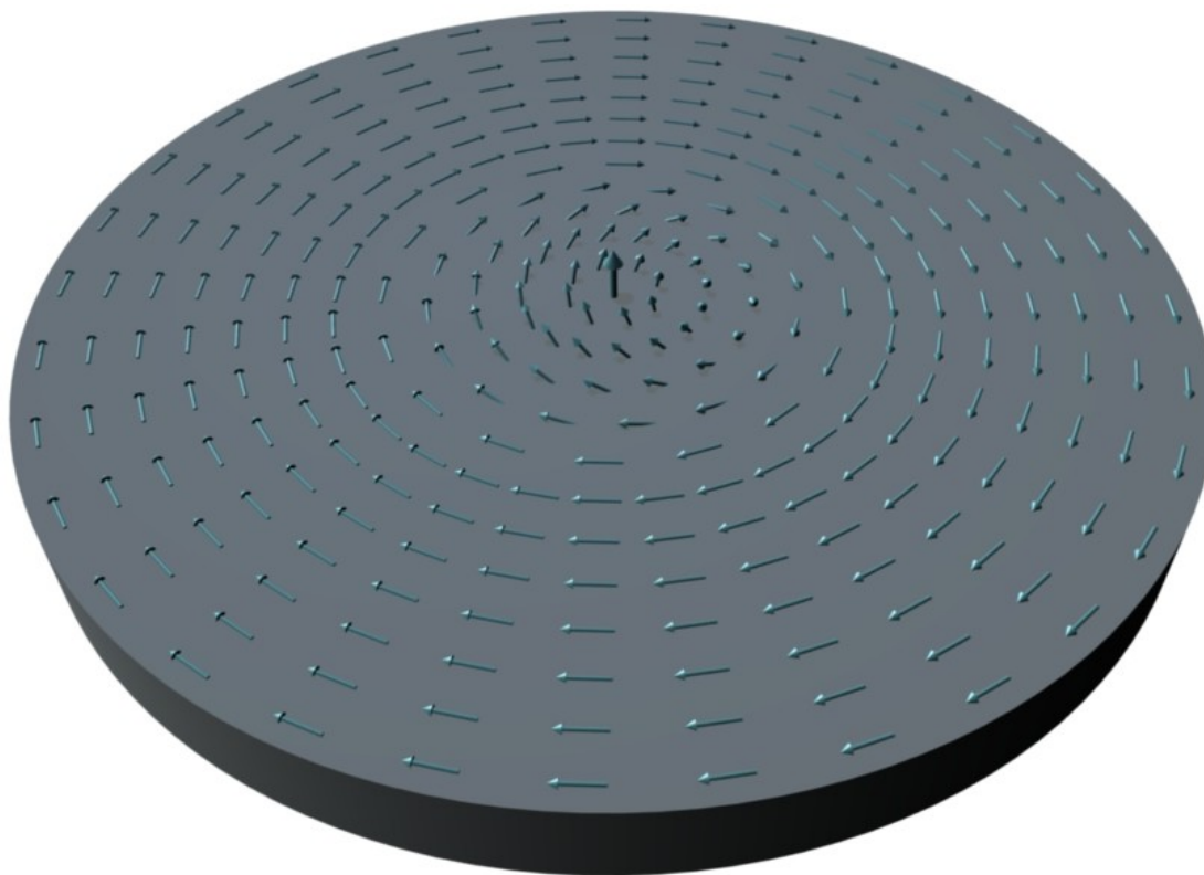
Figure 1.6 Magnetic vortex structure.
