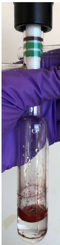
Figure 4.11 Ni- ISO CN-3 in an ampoule with 3 mL of Millipore water. The red sample floats on top and sticks to the walls of ampoule and does not mix with the water.
